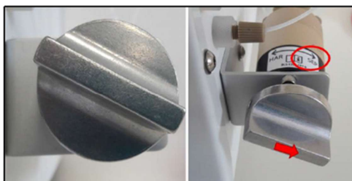
Figure 4 - Harvest/Separation valve returned to “SEP” position
