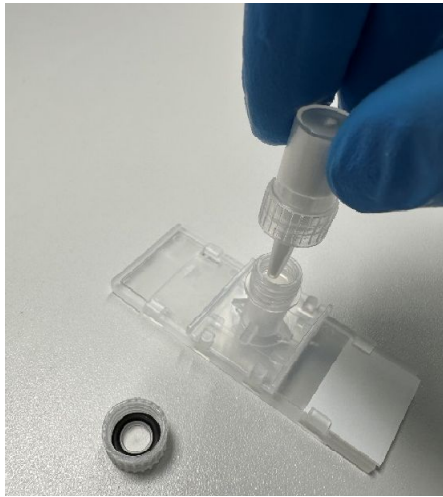
Figure 6a. Screwing on a CellKeep wicking cap.
