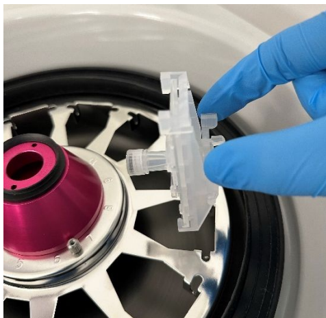
Figure 5a. Approaching the Cytospin 4 with CellKeep Cytospin adaptor side arms secure.
