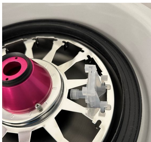
Figure 5c. The CellKeep Cytospin adaptor is locked into the Cytospin 4 slot.
