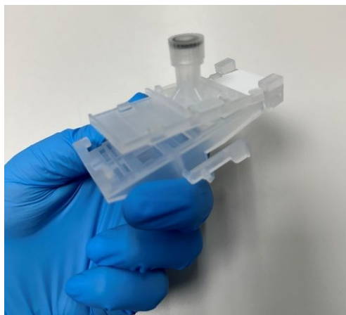
Figure 4a. Inserting the CellKeep slide through the CellKeep Cytospin adaptor upper brackets.
