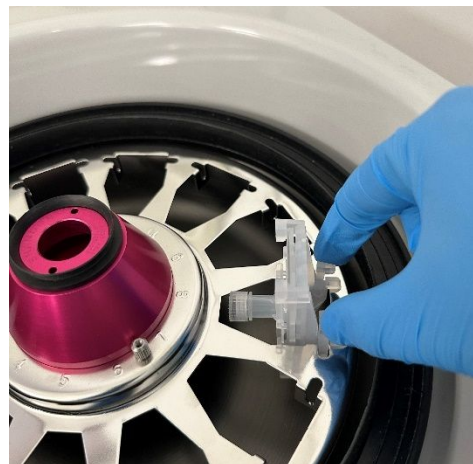
Figure 5b. Loading the CellKeep Cytospin adaptor into the Cytospin 4 slot.
