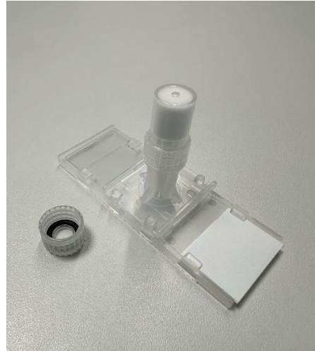
Figure 6b. CellKeep wicking cap attached.
