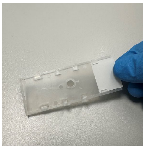
Figure 10a, b. Removing the microscope glass slide from the lower plastic casing.
