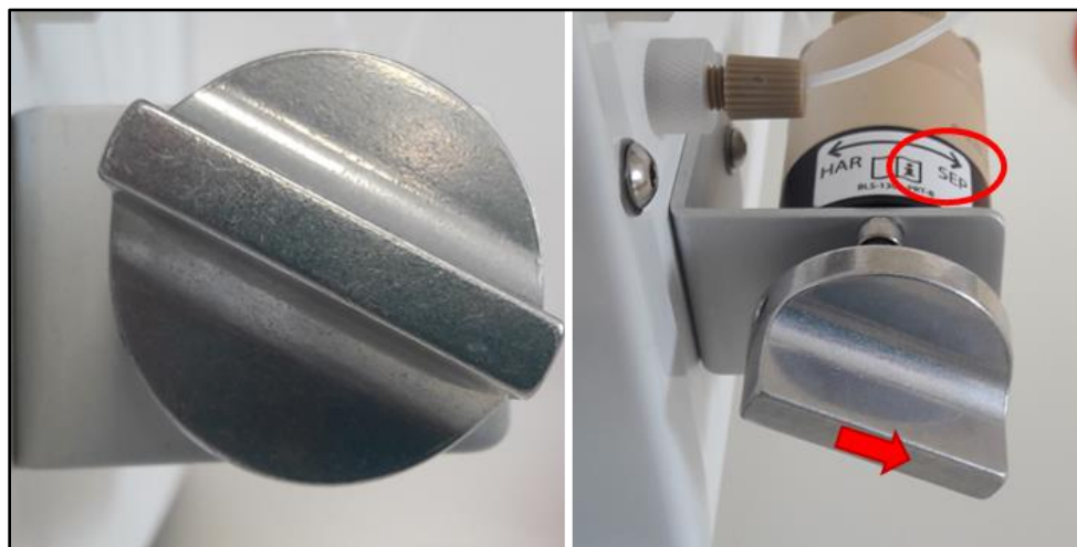
Figure 17. Harvest Valve in separation "SEP" position.
