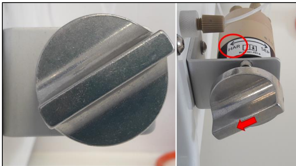
Figure 18. Harvest Valve in the harvest "HAR" position.
