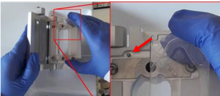
Figure 15a. Loading a Parsortix cassette into the clamp.
