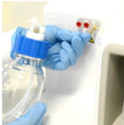
Figure 6b. Connecting the buffer reservoir.
