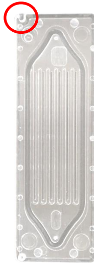
Figure 14. Parsortix cassette in correct orientation for loading into the clamp.
