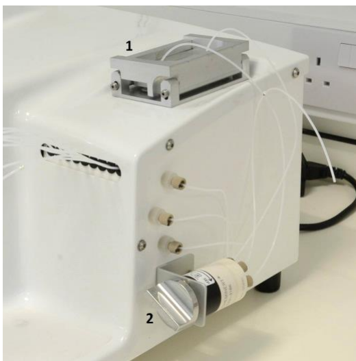
Figure 4. Cassette clamp (1) connected to the harvest valve (2). Figure 5. Rear view of the harvest valve.
