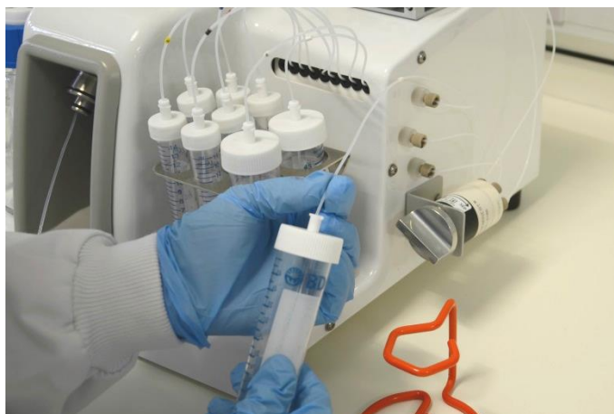
Figure 9. Connection of the harvest waste line to the waste tube.
